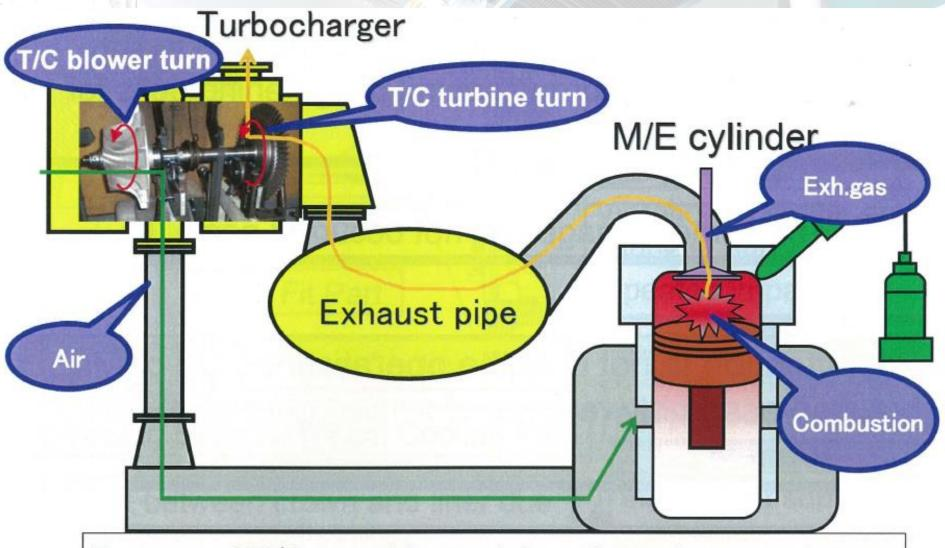
Purpose of T/C: send large air in order to increase output Damage to T/C ⇒ lead to speed reduction
