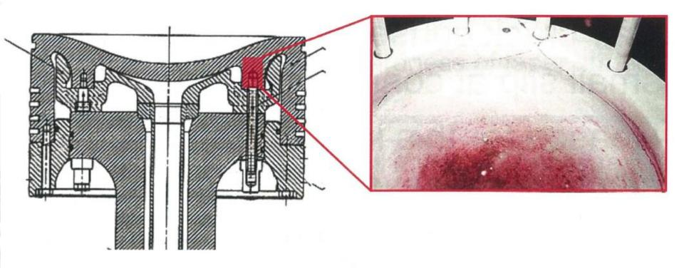
Two Cracks were found at piston head supporting part of M/E during a inspection
