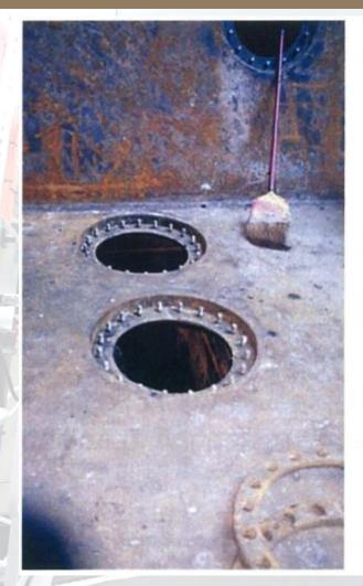
The manhole cover of bilge well that located between No.4 cargo hold and void space had not been tightened enough.
