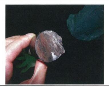
Section of bolt breakage (Crack is occurred at circumferential direction)
