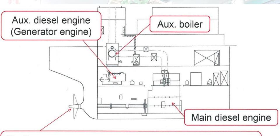
Shafting (Intermediate shaft / Propeller shaft / Propeller /Bearings)
