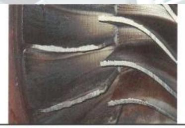
Blower Impeller (Reduction of 5 mm in thickness)
