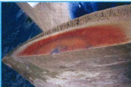
Fracture Surface of Blade "A"
