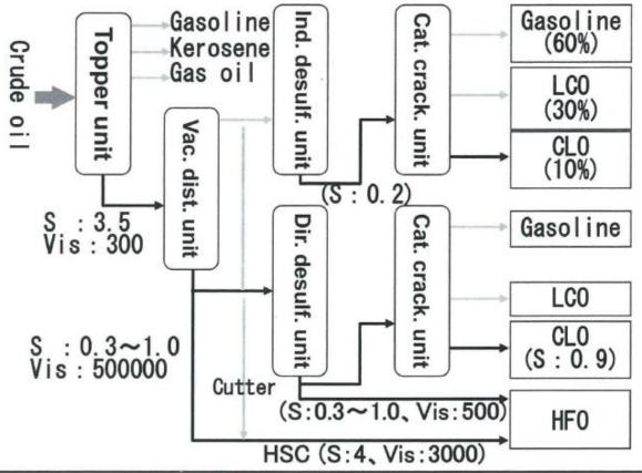
Note: FCC means Fluid Catalytic Cracking. In order to promote cracking reaction, they use powdered form catalyst which principal ingredients are alumina, silica.
