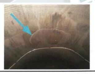
Crack on Cylinder Liner
