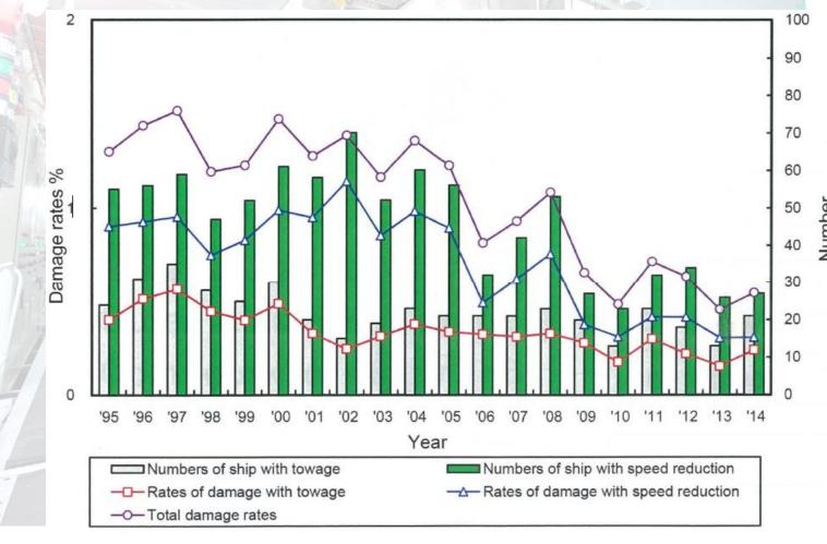
1. Introduction: Numbers and Damage Rates (Major Damage Breakdown)
