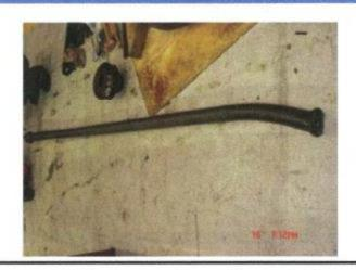
Bent Piston Cooling Pipe
