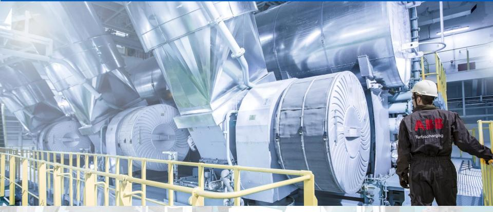
Send large amount of air to combustion chamber in order to increase engine output
