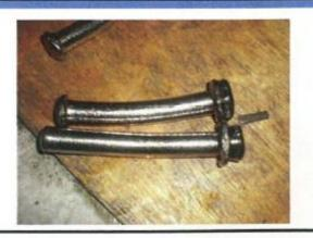
Bent Tightening Bolts for Piston Cooling Pipe
