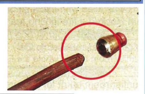
Over-tightening at installing
