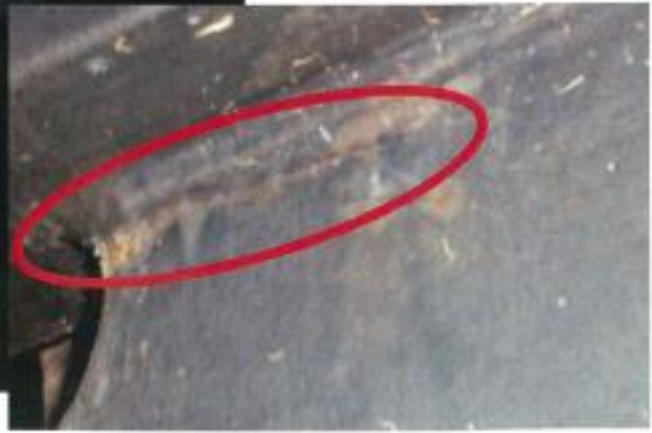
Crack in bracket on trance web at slot for bilge hopper longitudinal
